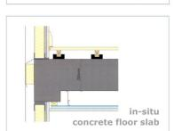
The Durabella Cradle System is designed for applications where the sub-floor is out of level tolerance or uneven and is an extension of the rinciple applied to the batten system. Durabella Cradle & Batten systems have the ability to resist compression under load whilst providing a continuing level of sound insulation. The cradle system is particularly effective in overcoming difficult site problems and can be laid with an overall depth between 55mm and 500mm.
